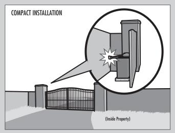
The illustration is an example of a compact installation. If the operator arm will hit an obstruction when the gate is in the open position follow the directions for Compact Installation.
