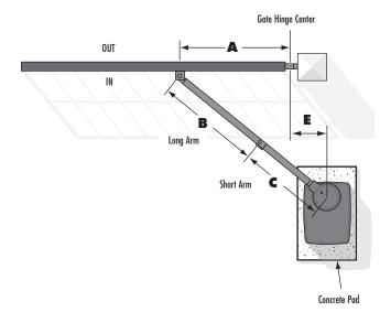
Dimension (A) thru (E) are from the center of one pivot point to the center of another pivot point.
