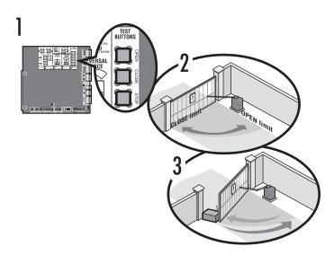
Open and close the gate with the TEST BUTTONS, ensuring that the gate is stopping at the proper open and close limit positions.
