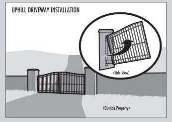
The illustration is an example of an uphill driveway installation. If installing the operator on a hill, a special swivel arm and hinges are required (not provided).
