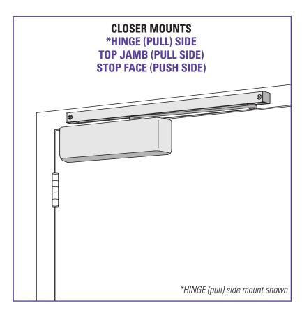
The 4040T SMOOTHEE® is LCN's most flexible heavy duty track closer designed specifically for interior doors in institutional and other rugged high traffic applications.
